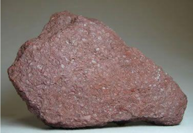
Plate vii: Iron Ore is a chemical sedimentary rock that forms when iron and oxygen (and sometimes other substances) combine in solution and deposit as a sediment.
