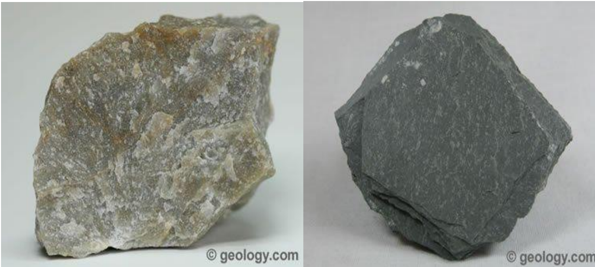
Plate viii: Quartzite is a non-foliated metamorphic rock produced by metamorphism of sandstone. Plate ix: Slate is a foliated metamorphic rock produced by metamorphism of shale.
