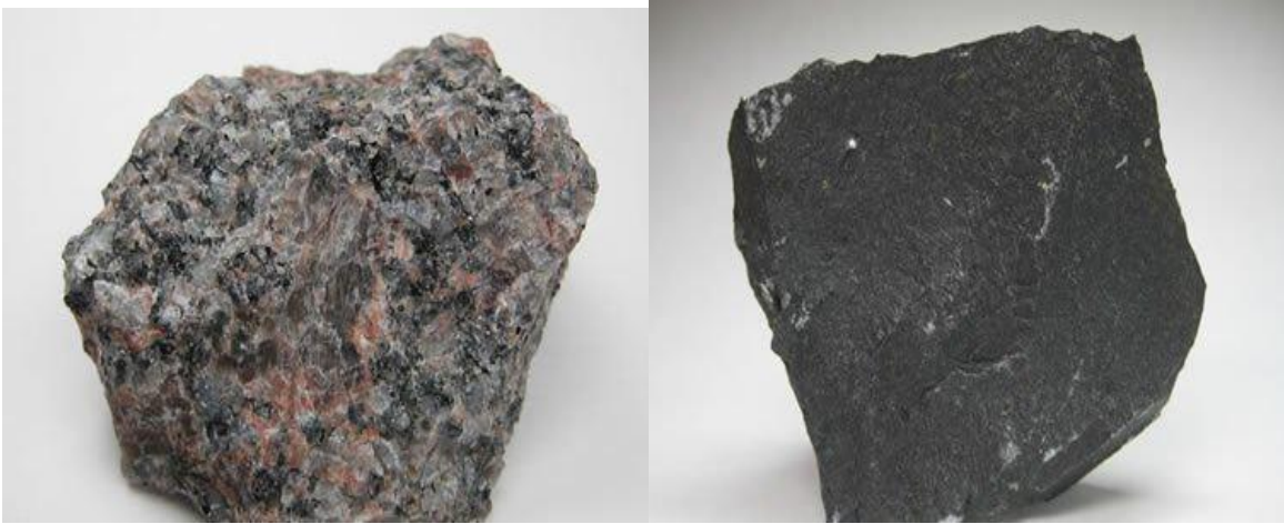
Plate i: Granite is a coarse-grained, light-colored Intrusive igneous rock Plate ii: Basalt is a fine-grained, dark-colored Extrusive igneous rock
