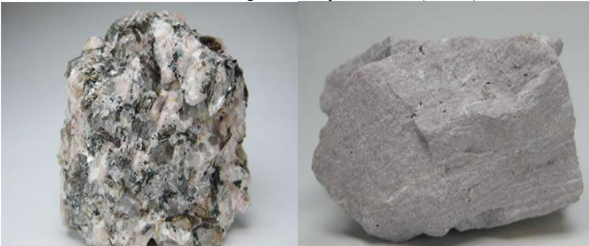
Plate iii: Pegmatite is a light-colored, extremely Coarse-grained intrusive igneous rock. Plate iv: Rhyolite is a light-colored, fine-grained Extrusive igneous rock.
