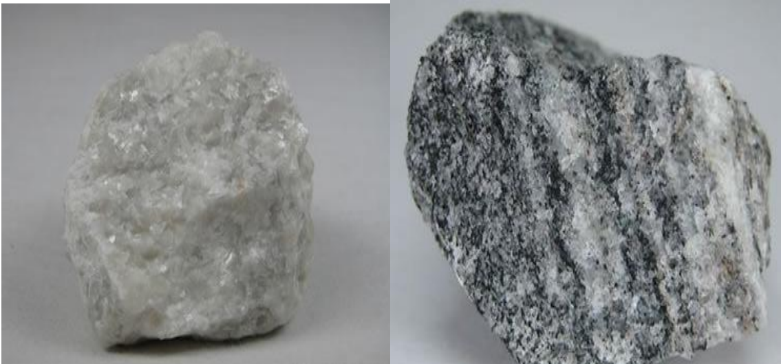
Plate x: Marble is a non-foliated metamorphic rock produced by metamorphism of limestone. It has a granular appearance and is made up of calcium carbonate mineral grains. It typically contains abundant Quartz or feldspar minerals. Plate xi: Gneiss is a foliated metamorphic rock that produced by metamorphism of granite. It has a banded appearance and is made up of granular minerals. It is composed of calcium carbonate mineral grains. It typically contains abundant Quartz or feldspar minerals.
