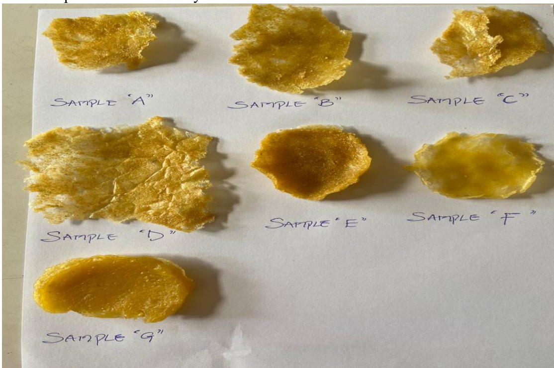
Plate 2: Pictorial representation of bioplastics produced from maize cob of different samples
