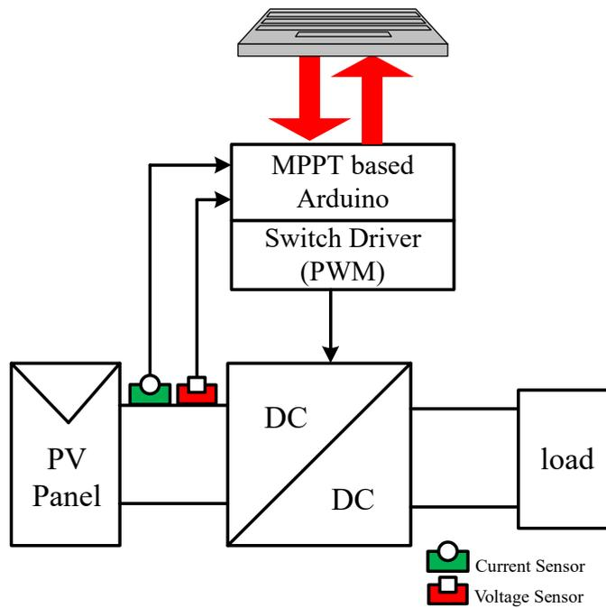
Fig 8. Block diagram of the proposed setup
