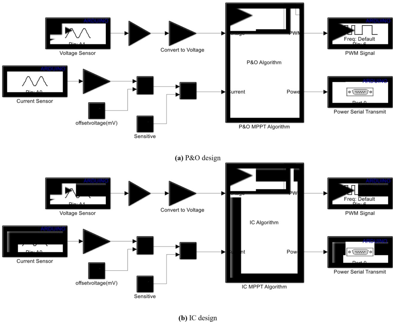
**Fig 5.** The algorithms design with Simulink support package for Arduino hardware
