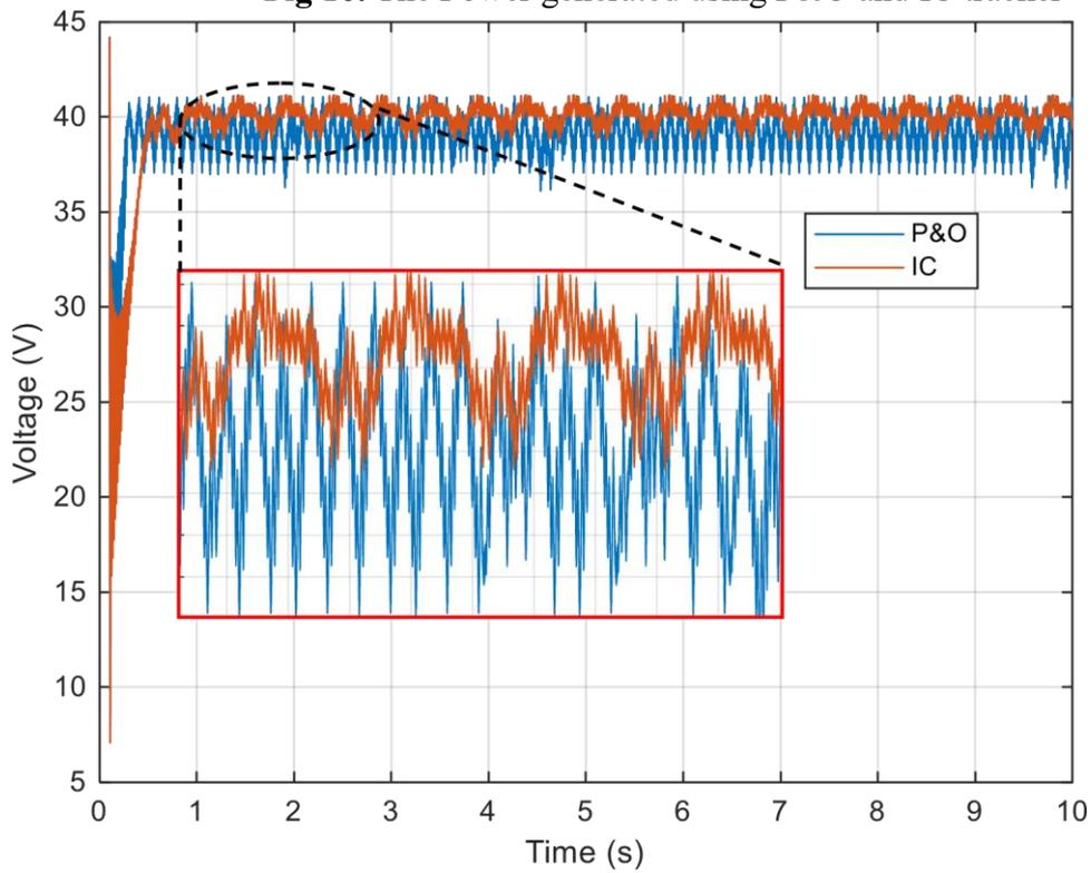
**Fig 11.** The voltage waveform of PV panel
