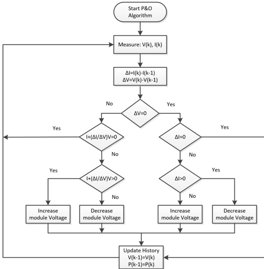
**Fig 4.** The flowchart of Incremental Conductance
