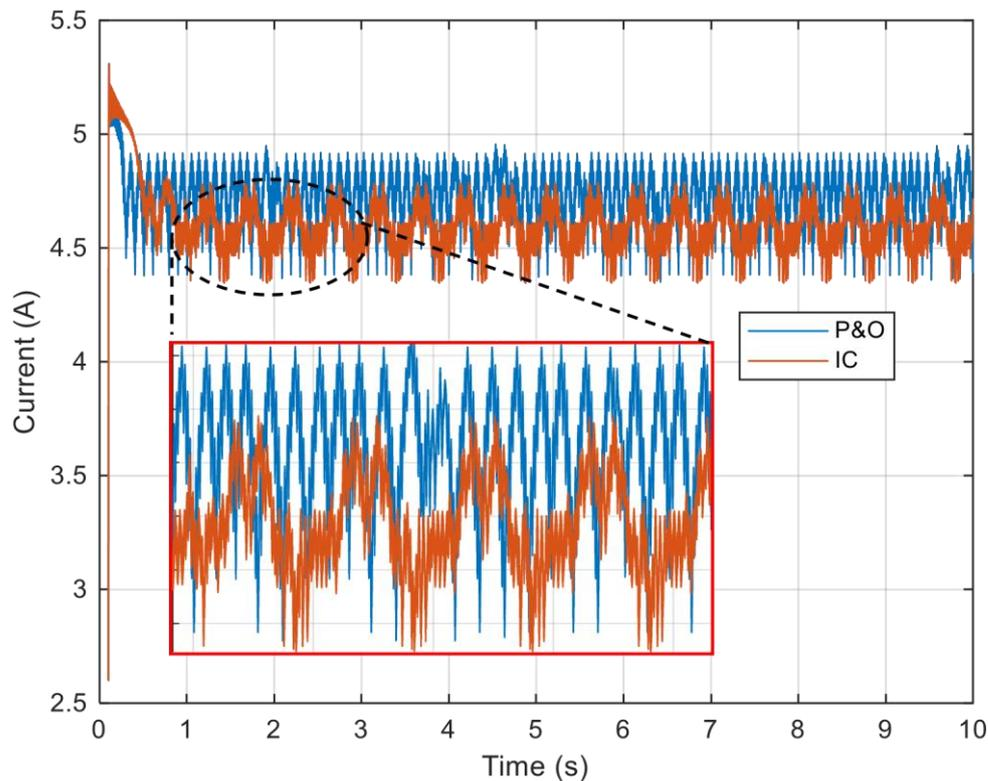
Fig 12. The current waveform of PV panel
