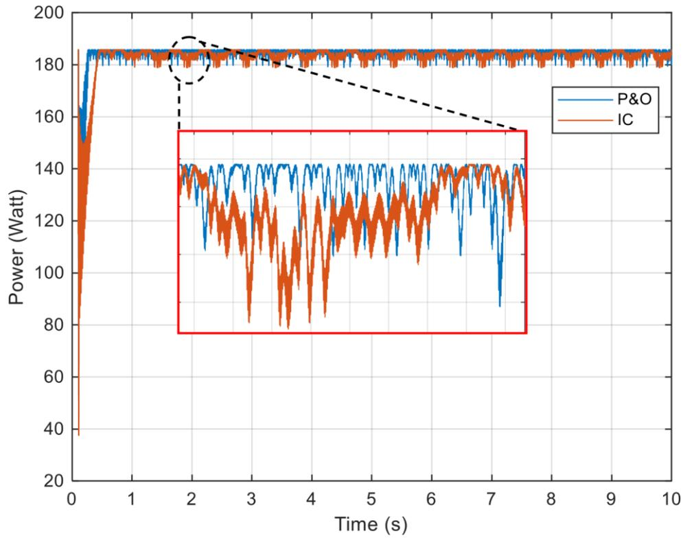
**Fig 10.** The Power generated using P&O and IC tracker
