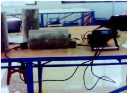
Fig 3. Ultrasonic pulse velocity setup
