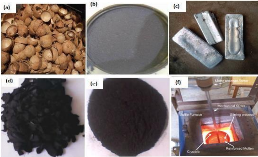
Figure 1: (a) Coconut shells (b) Silicon carbide (c) Cast AA6061 ingot (d) Crushed carbonized coconut shells (e) Carbonized coconut particulates (f) Stir casting furnace
