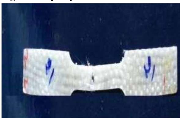
Fig 7.2 Sample specimen of S glass-Epoxy
