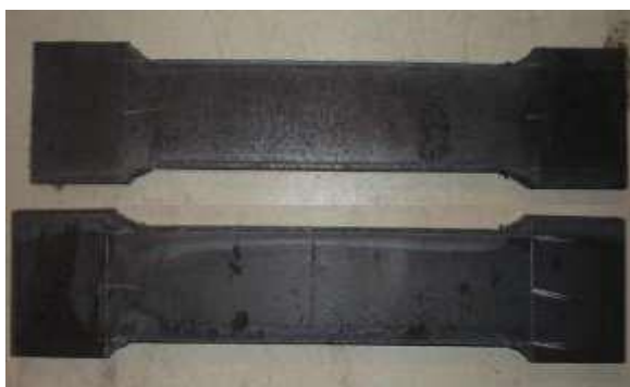
Fig 7.1 Sample specimen of EN45 Steel
