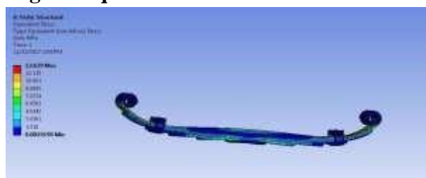
Fig 8.2 Equivalent stress of composite leaf spring
