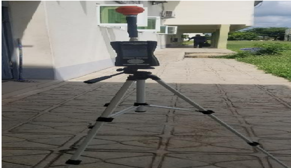
Figure 3. Photograph of the RF meter mounted on a tripod stand
