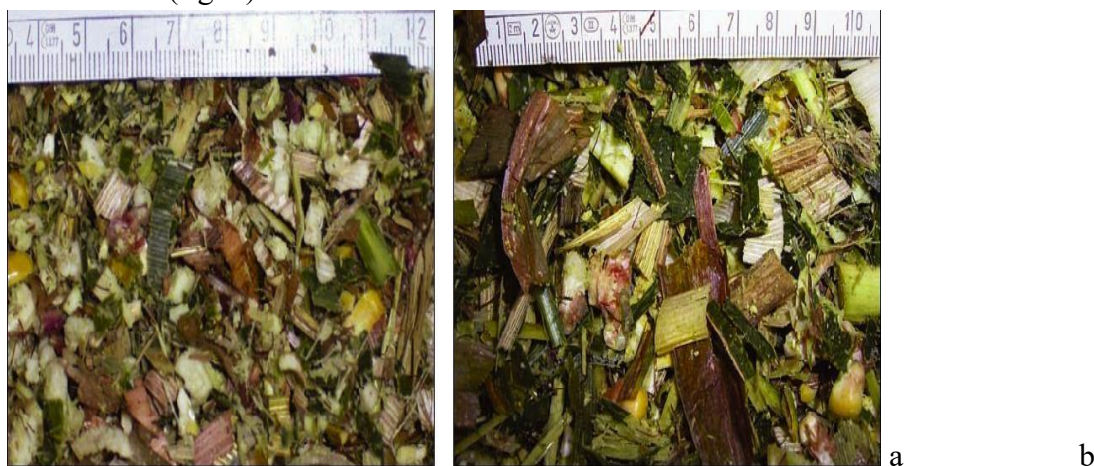
Fig. 5. Shredded mass with a theoretical rod length of 5 mm (a), with a theoretical rod length of 20 mm (b)
